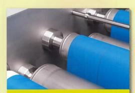
Press rollers on fixed shafts with encapsulated roller bearings no alternating bending stress
